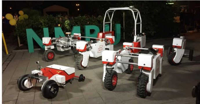
Figure 16. Different examples of robots assembled from Thorvald II modules
