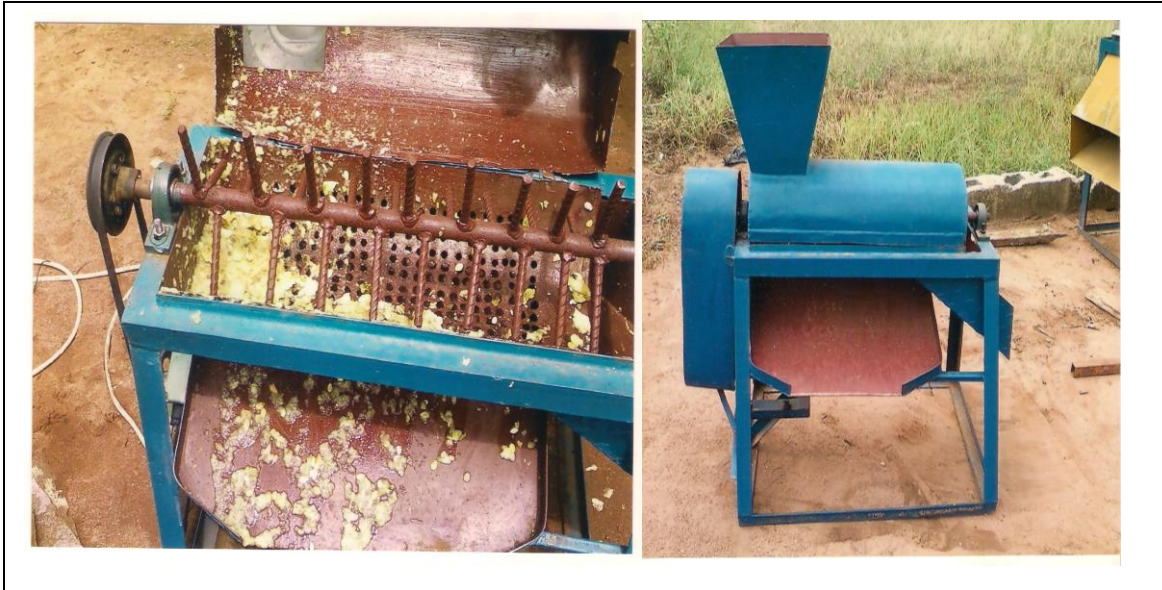
Figure 1: Pictorial view of the melon depodding machine.
